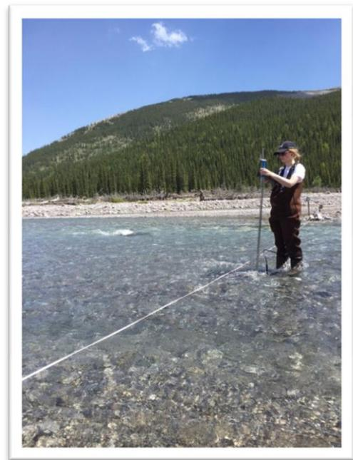
NSERC Undergraduate Research Assistantship holder Carly Doig takes measurements for velocity/depth to determine surface discharge of the Big Elbow.
