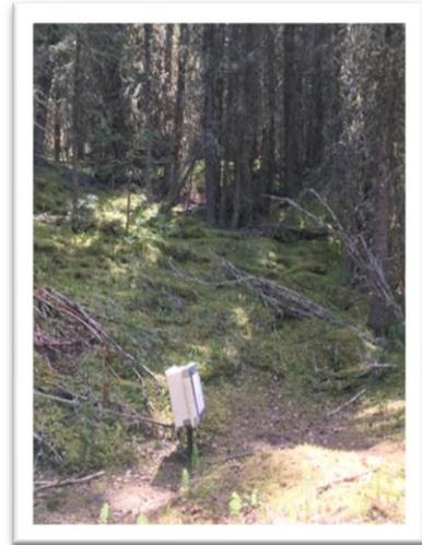
A piezometer measures groundwater levels at the base of the Forgetmenot Ridge.
